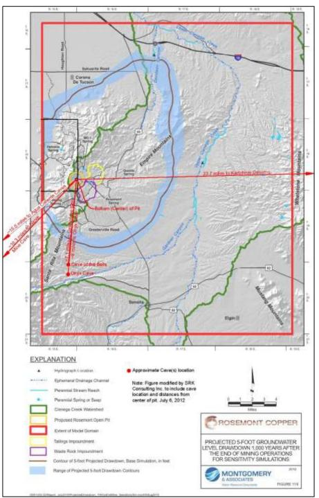
Figure 6 Location of significant cave resources in the Santa Rita Mountains (modified from M&A 2009 figure showing steady state (1,000 years) groundwater drawdown contours)
