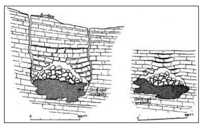
Figure 3 Subsidence features in thin-bedded limestone, near surface (left) and at depth (right) (Wisser, 1927, Figs. 7, 8)
