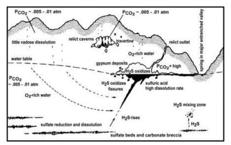
Figure 4 Origin and typical distribution of caves formed by oxidation of hydrogen sulfide (Palmer, 2000)
